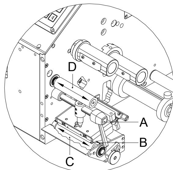
A soiled print roll can lead to reduced print quality and can affect transport of material.
